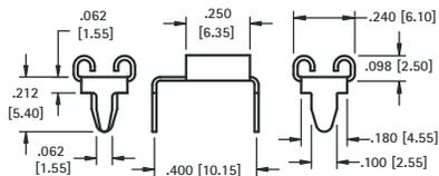
CAT. NO. 3550-2 Tin Plate UL Current Rating: 20 Amps @ 500V AC
