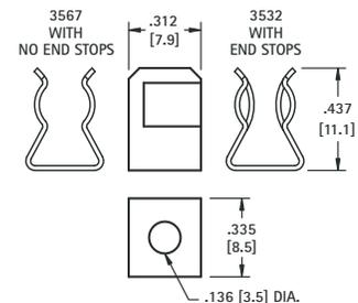
\*Fuse clips without end stops are not UL recognized
